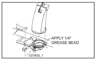
Figure 16. Apply Grease to Discharge Chute Ring
